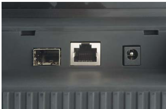
Figure 3-3 Power and Input/Output Ports
