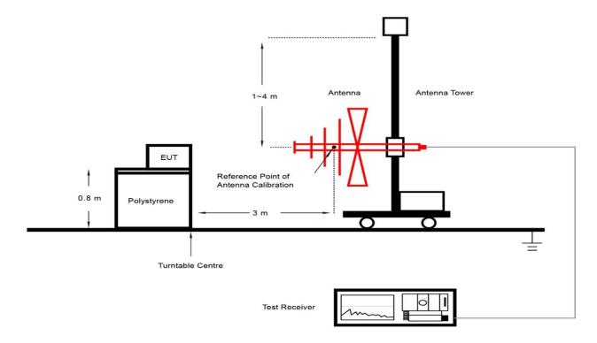
Above 1GHz Test Setup:
