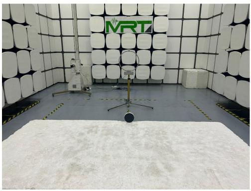
Description: Radiated Spurious Emission Test Setup for Below 30MHz
