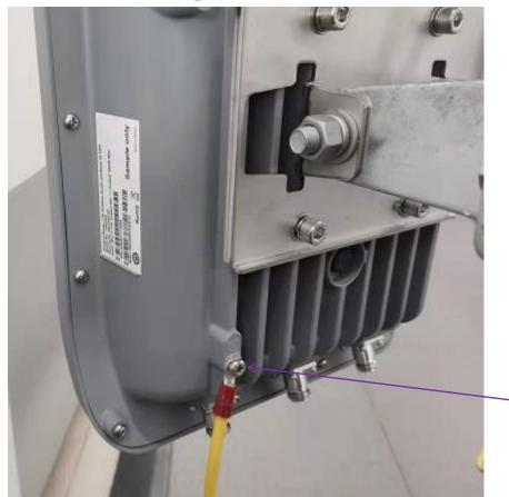
Grounding screw on the device
