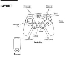
**Antenna Receiver:** Used to transmit and receive data from the controller to the game console.
