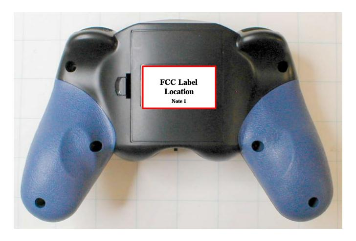
Note 1: The manufacturer attests that the unit will not operate without the battery compartment cover in place.
