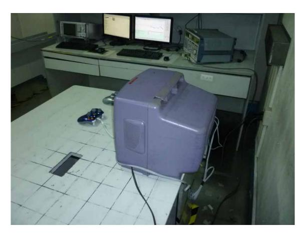
Photos of Radiated Emission Test (In Anechoic Chamber)
