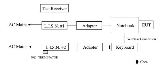
(EUT: Eclipse Wireless Litetouch Keyboard (Dongle))
