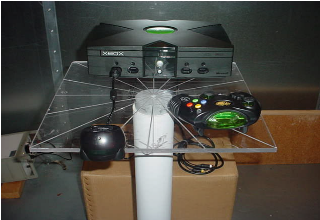
Photo of setup during Conducted Emission testing, showing the X-Box and the Base Unit, along with the Game Controller for normal duplex operation.
