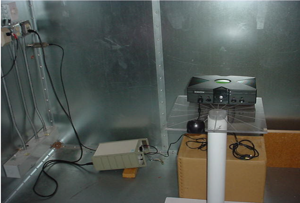
Conducted Emission Setup Overview
