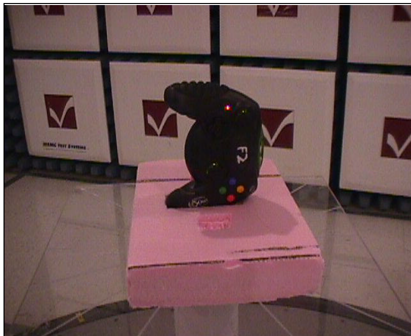
View of the EUT, as setup during radiated emissions tests, shown on side orientation for worst-case emissions.
