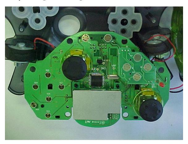
2.4 GHz wireless controller for X-Box Video Game System 2408.448 – 2476.032MHz Digital Radio
