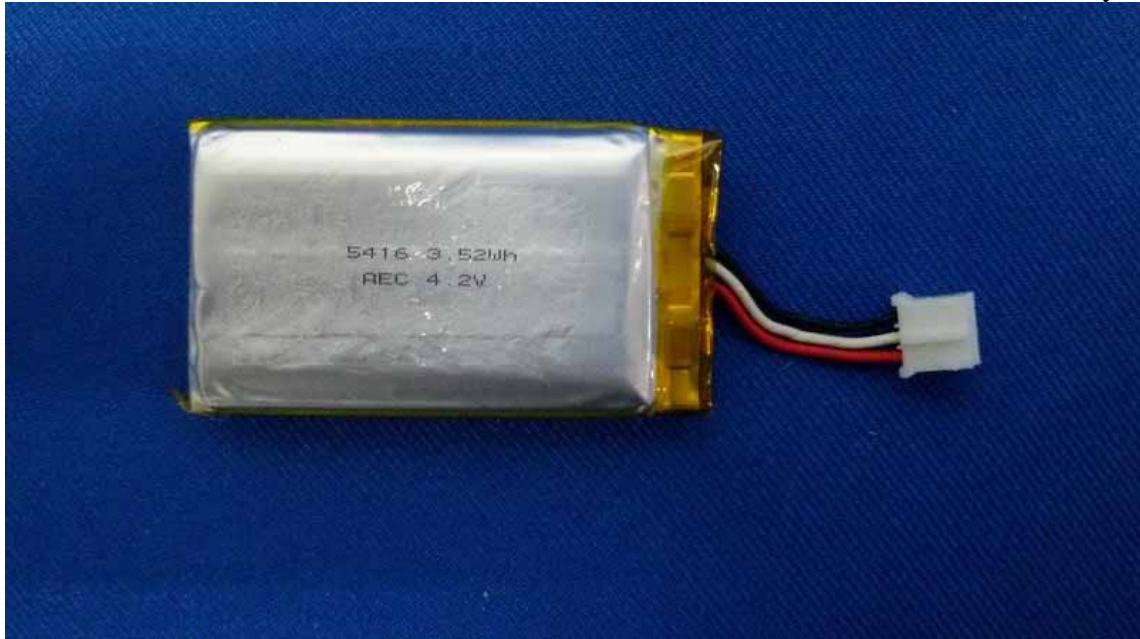
Figure 13 Battery of the EUT
