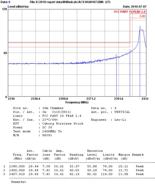
1. Emission Level= Antenna Factor + Cable Loss -Amp Factor + Reading.
