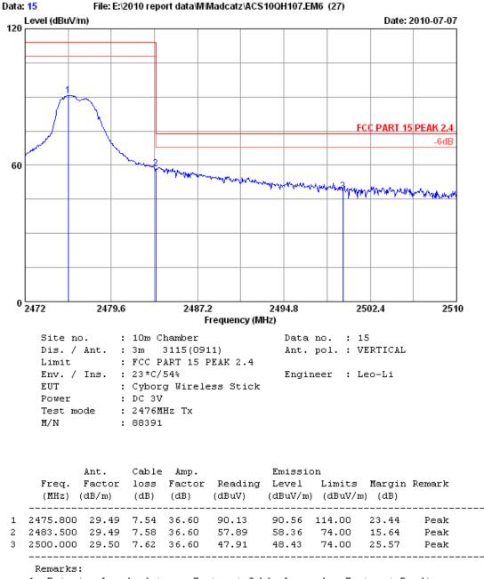
1. Emission Level= Antenna Factor + Cable Loss -Amp Factor + Reading.
