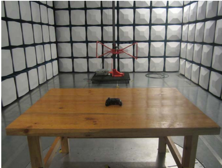
Radiated Emission View – above 1 GHz
