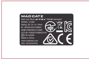
Rating Label (Size: 24.6mm x 14.6mm) White graphic on black background Laminate Matt PP film on top (過啞膠)
