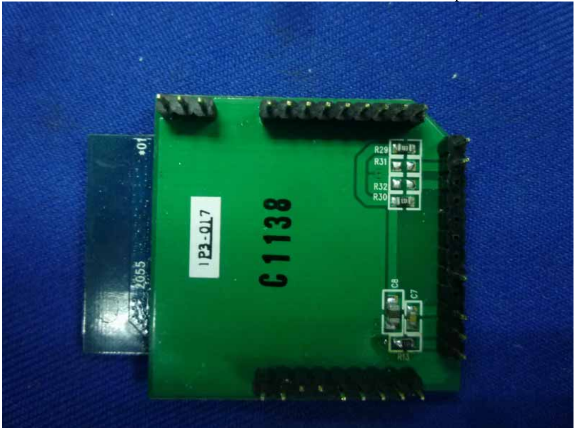
Figure 12 Component Side of the PCB
