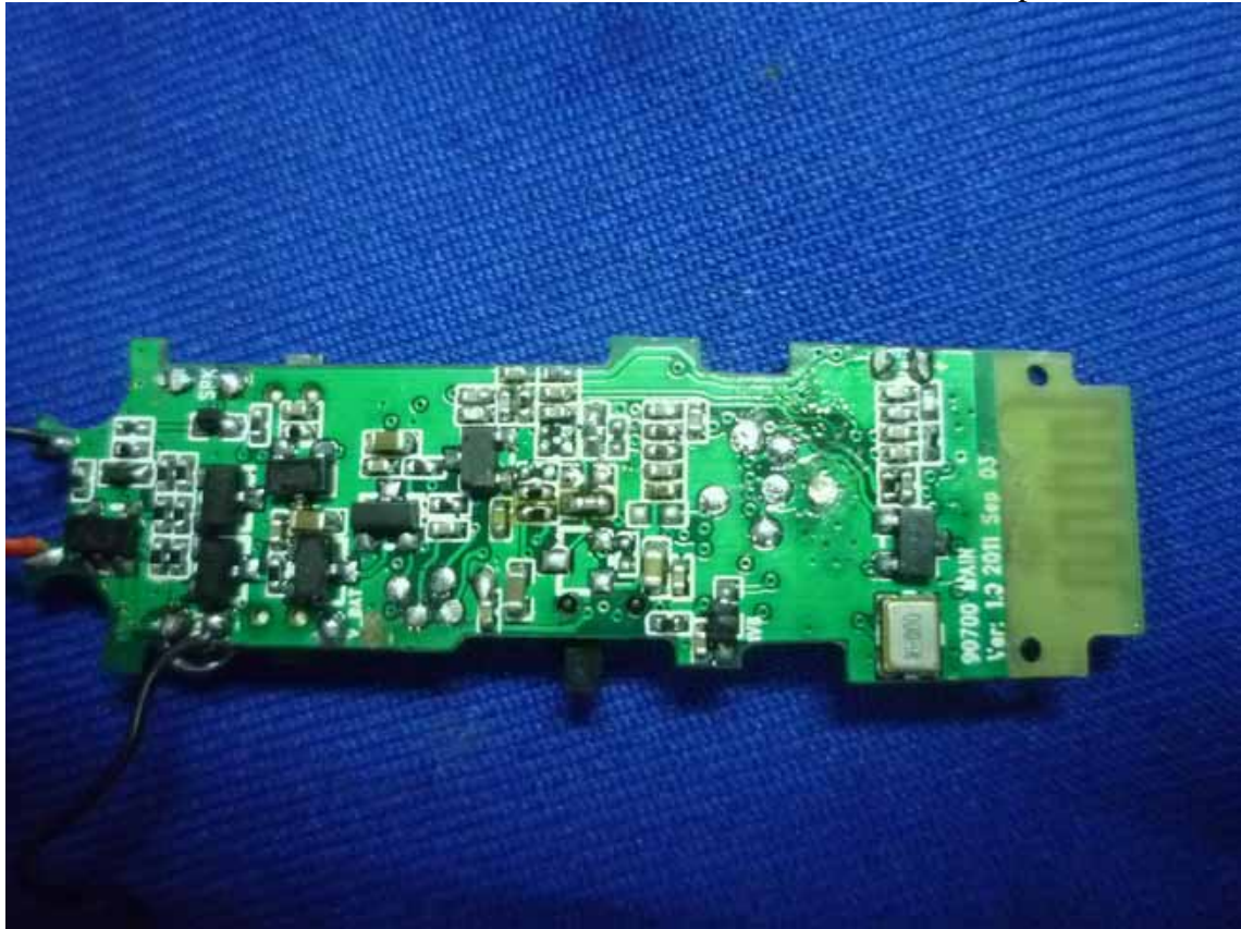
Figure 17 Components Side of the PCB
