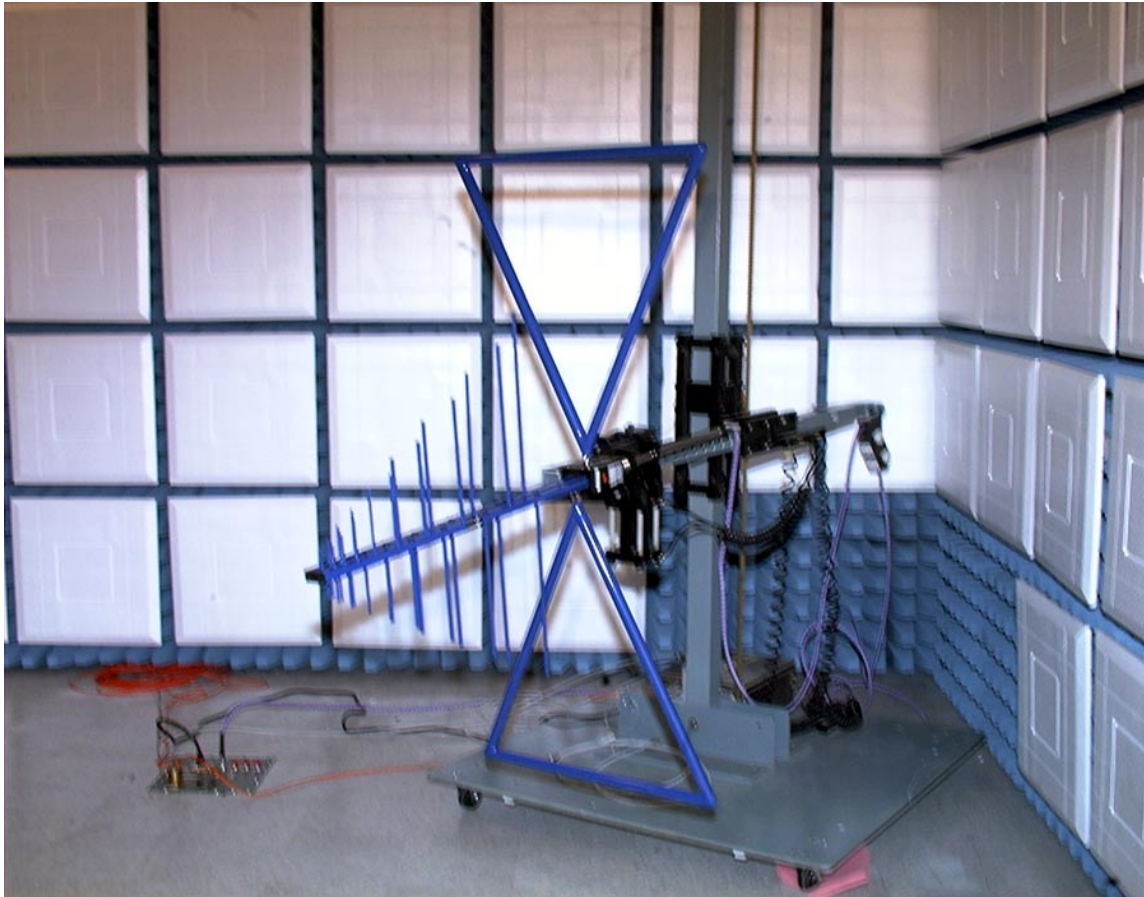
Figure 12.13 Radiated Emission 30MHz - 1GHz Test Setup
