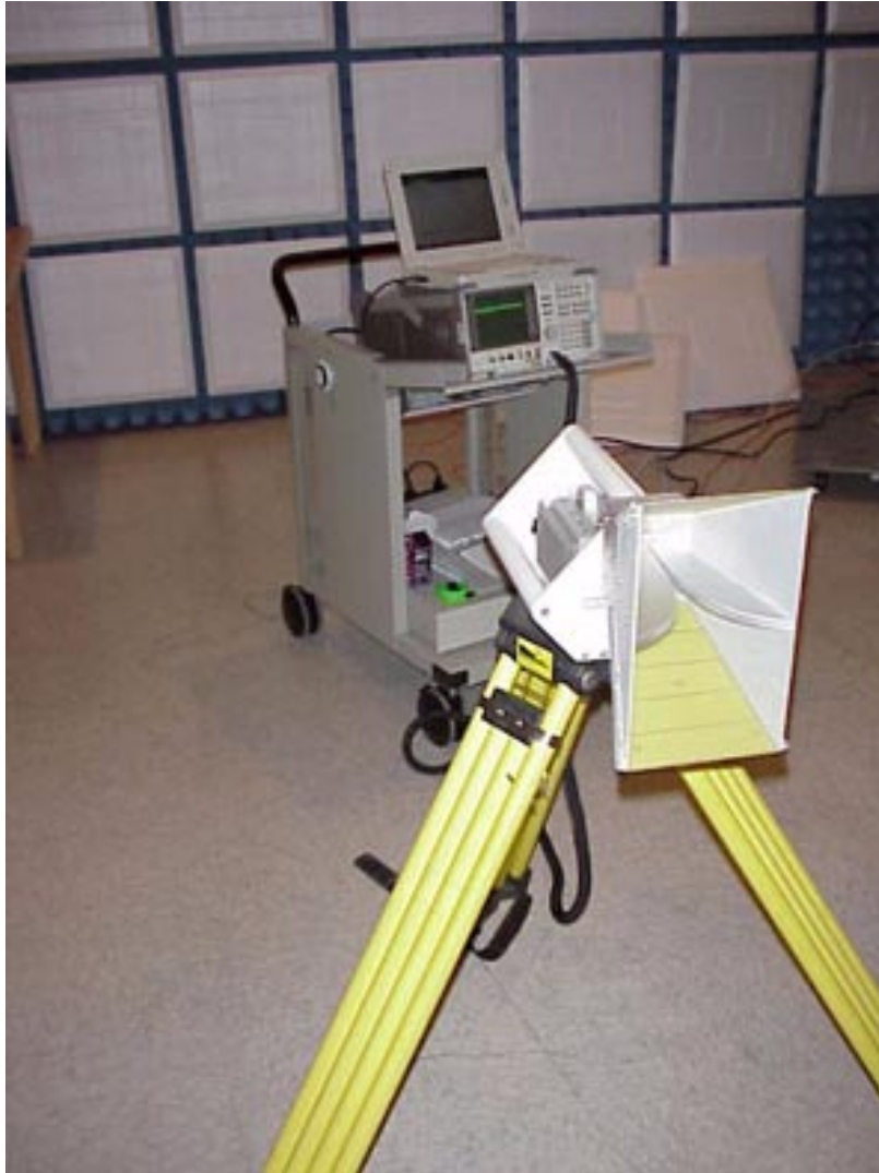
Figure 12.12HP 84300A E62 Microwave Intentional Radiator System
