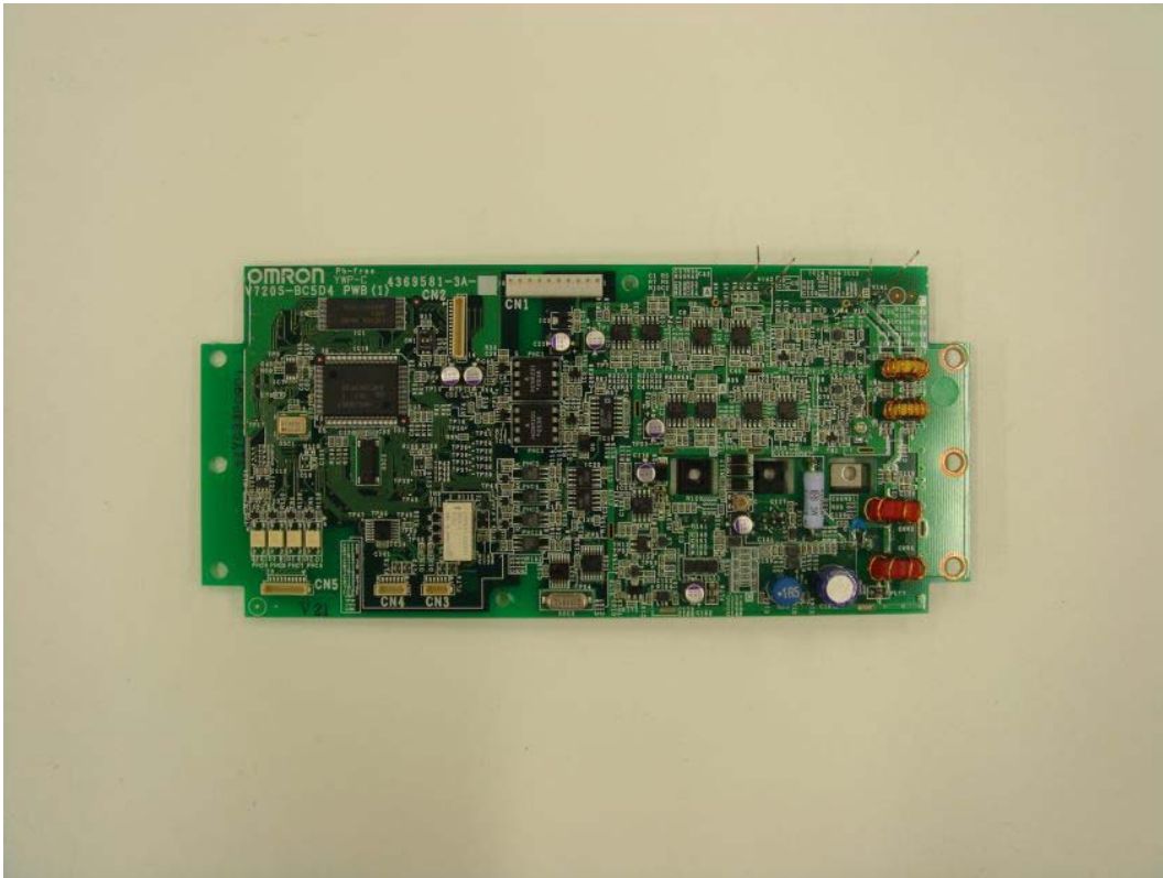
Controlling wireless board (Front)
