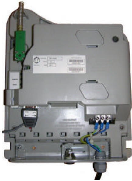
Figure 1 The XR-3100 serial port with the DT-100 Cross band programming cable attached.
