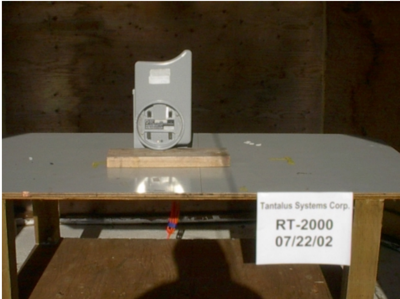
Emissions Test Setup Front View
