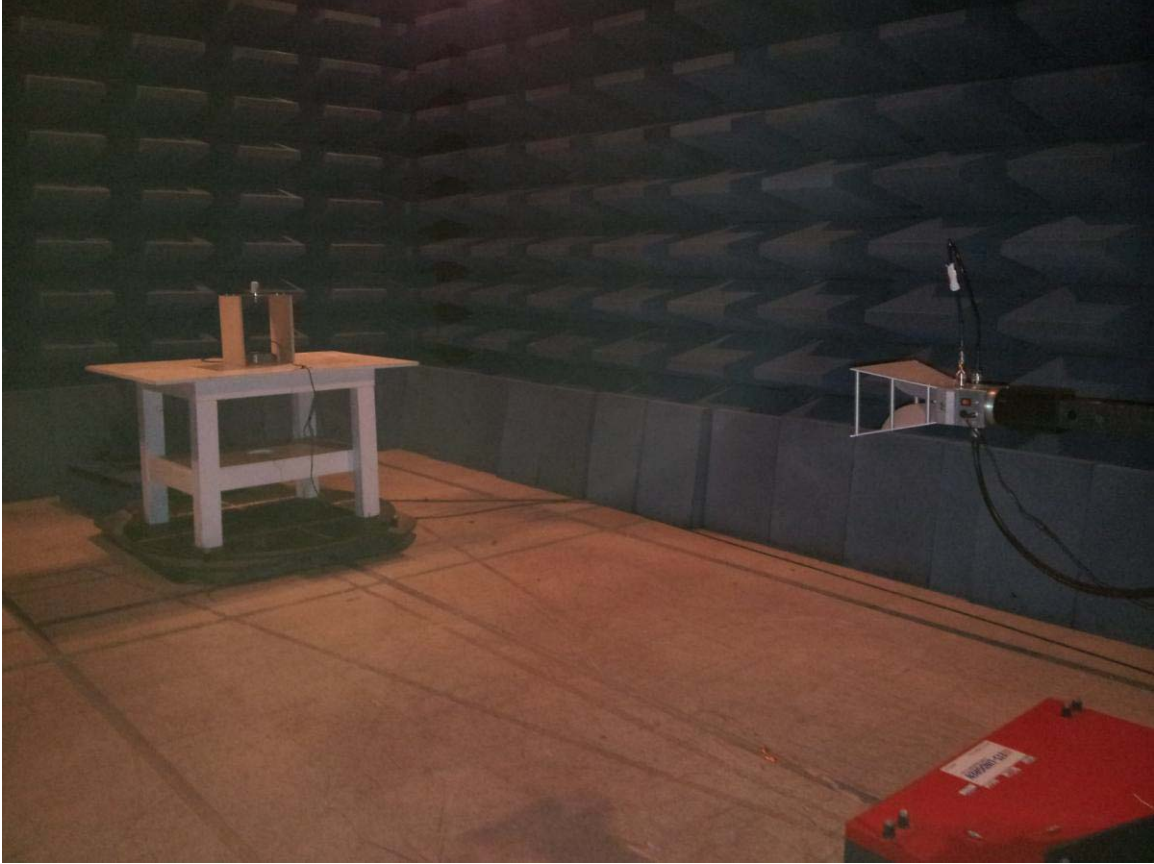
Emissions Test Setup – Intentional/Unintentional Radiated Emissions 1000 - 10000 MHz
