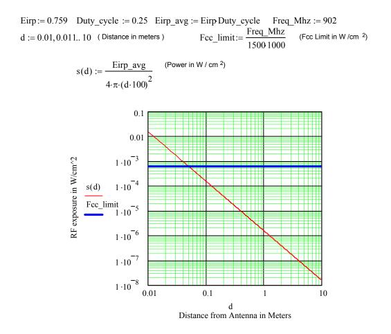
From the graph, it can be observed that the distance at which the RF exposure would exceed the limit would be 6.2cm. The far field distance for a small antenna is given by any distance greater than  $\lambda/2\pi$ ; this equates to a minimum distance of 5.3cm, therefore this calculation is valid.
