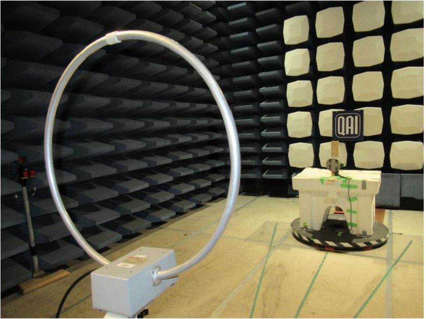
Emissions Test Setup – Unintentional Radiated Emissions 10kHz – 30MHz
