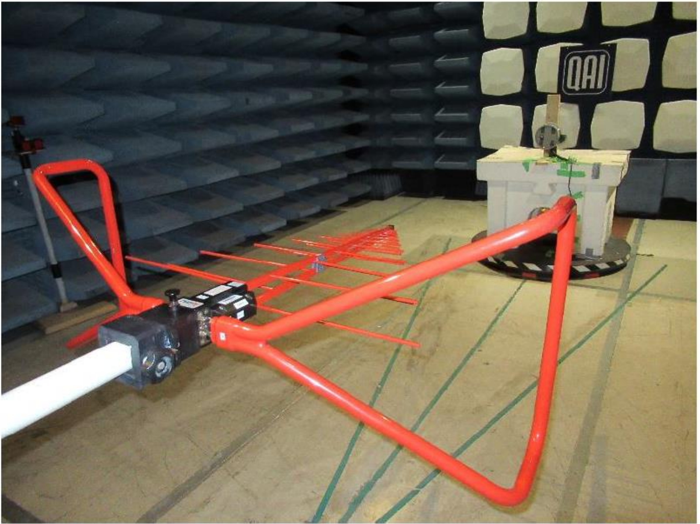
Emissions Test Setup – Unintentional Radiated Emissions 30 – 1000MHz
