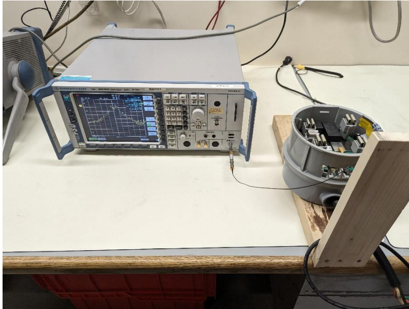
Figure 91: Conducted RF Measurement Setup
