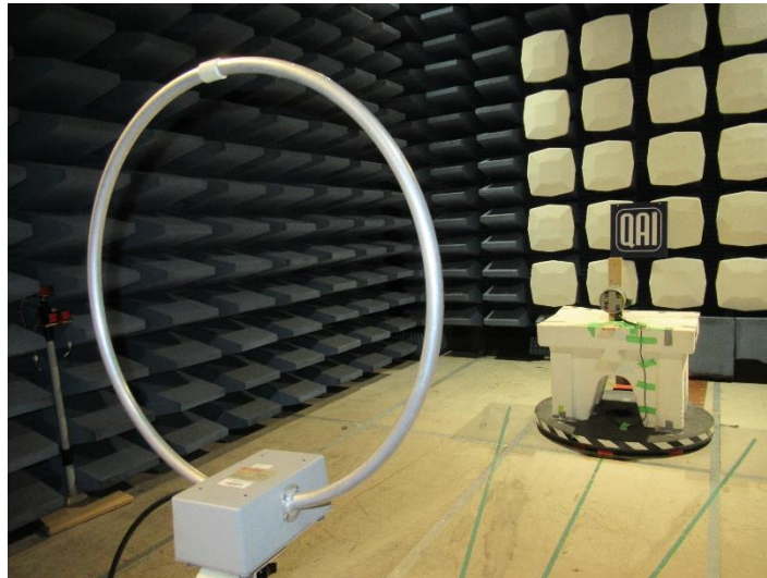
Figure 93: Radiated Measurement Setup, < 30 MHz
