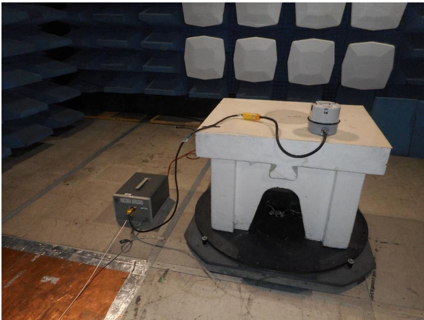
AC conducted Emissions Test Setup
