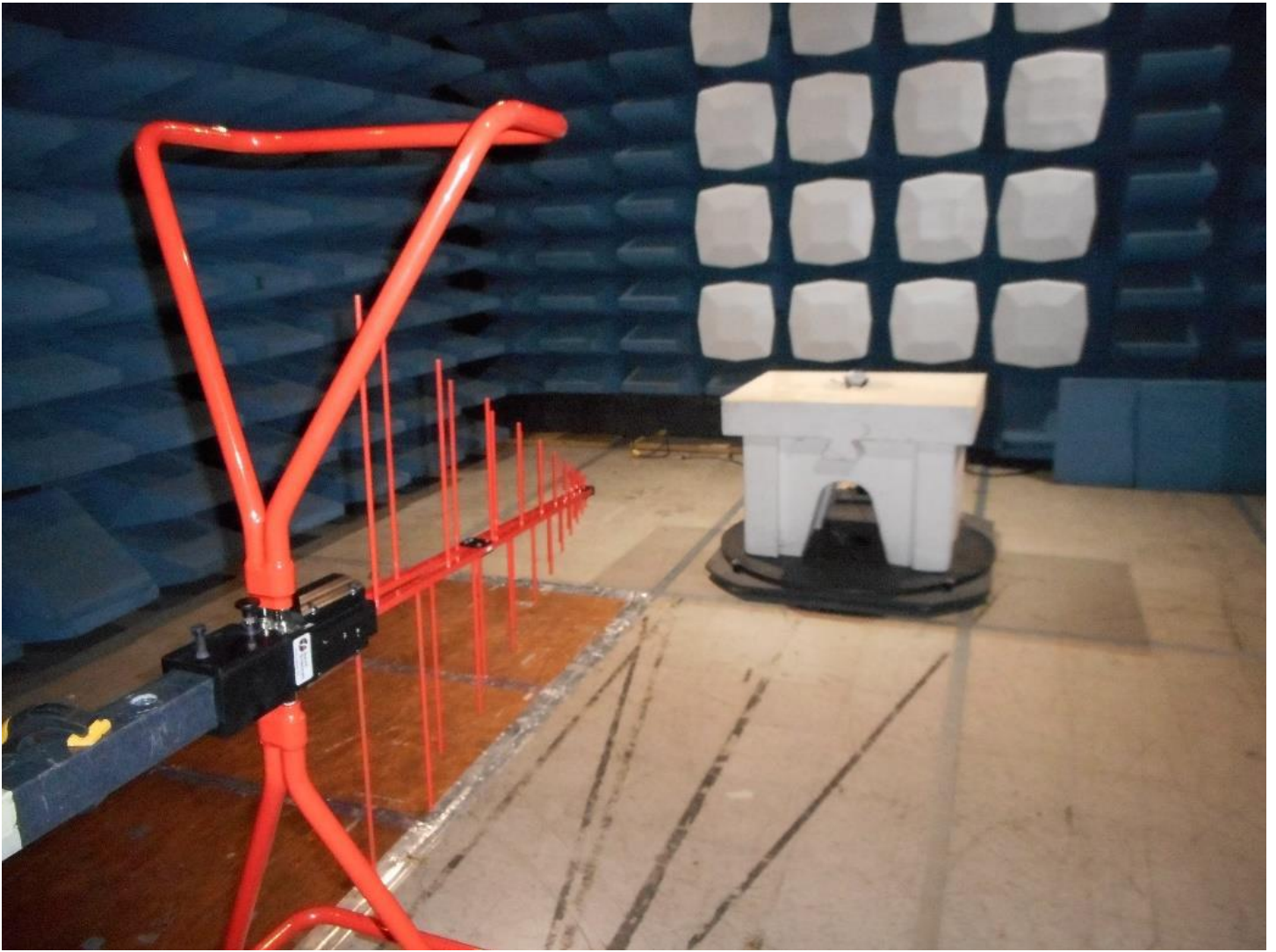
Emissions Test Setup – Intentional Radiated Emissions 30 – 1000MHz
