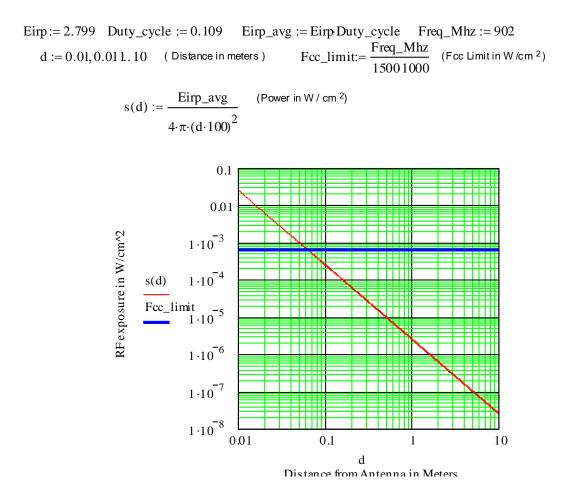
From the graph, it can be observed that the distance at which the RF exposure would exceed the limit would be approx. 6.5cm. The far field distance for a small antenna is given by any distance greater than  $\lambda/2\pi$ ; this equates to a minimum distance of 5.3cm, therefore this calculation is valid and so the minimum distance must be 6.5cm.
