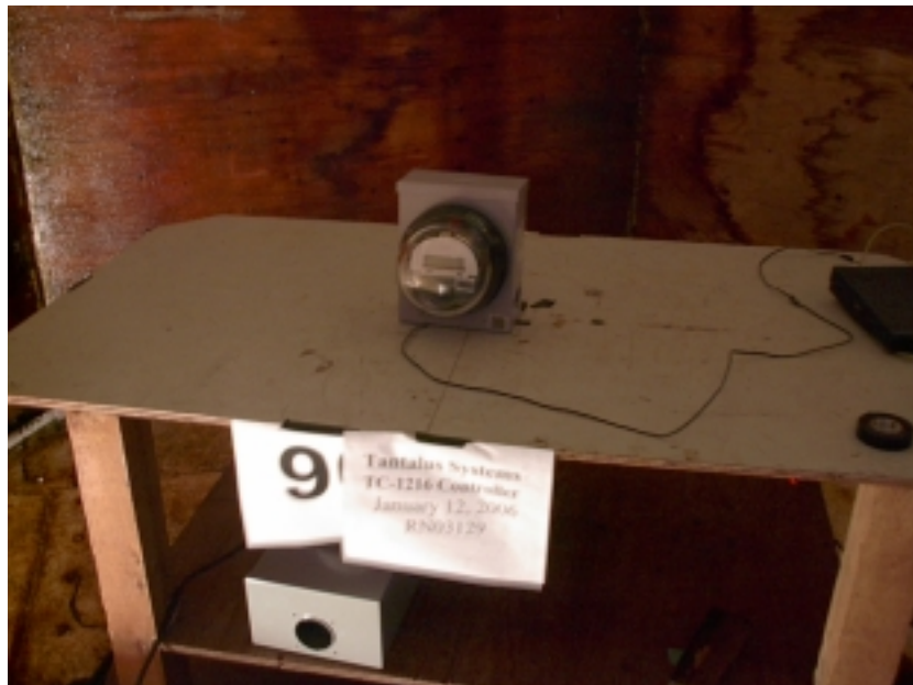
Emissions Test Setup for Conducted Emission
