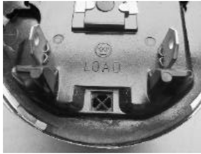
Figure 2: ABB AB-1 Vent hole with “crosshairs”.
