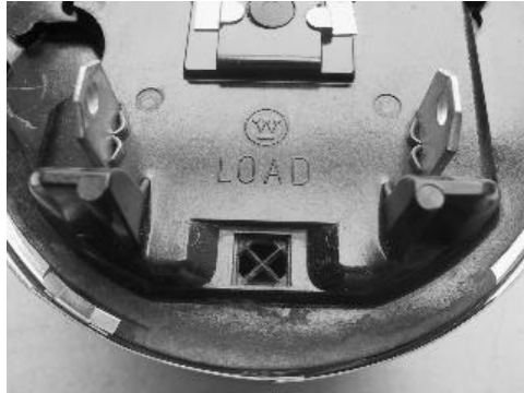
Figure 2: ABB AB-1 Vent hole with “crosshairs”.
