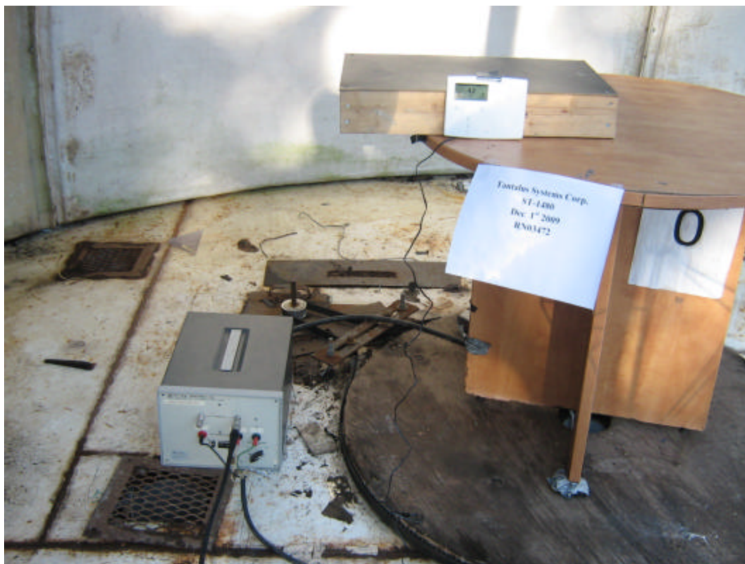
Figure 17 - AC Conducted Test Setup - Front View
