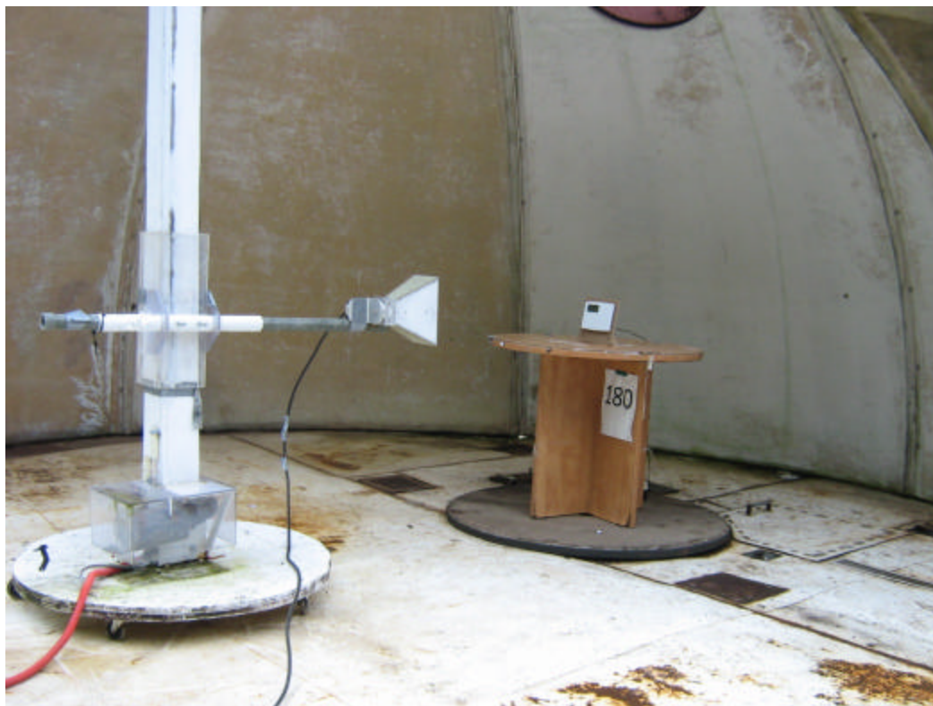
Figure 18 - Emissions Test Setup – Radiated Emissions
