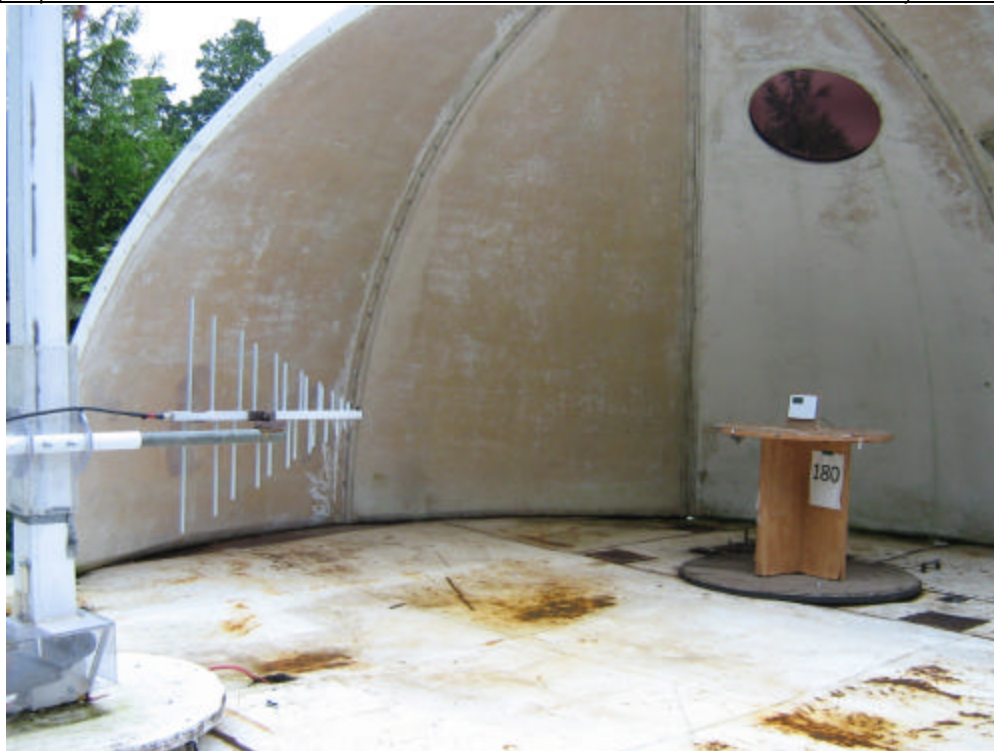
Figure 19 - Emissions Test Setup – Unintentional Radiated Emissions
