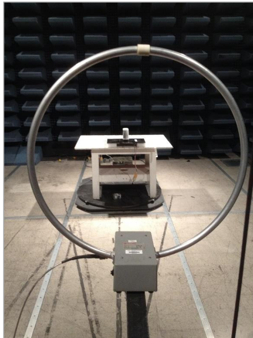
Figure 2: Radiated Emissions (below 30MHz) Test Setup
