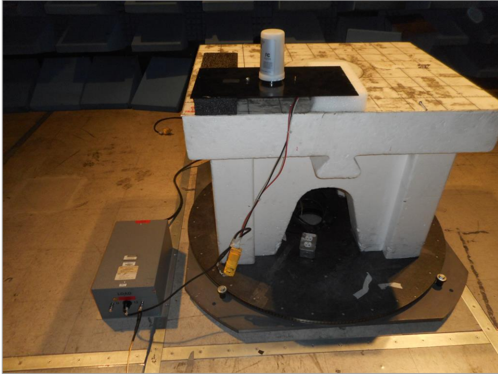
Figure 5: Conducted Emissions Test Setup
