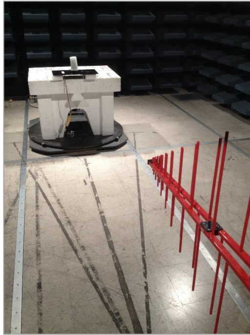
Figure 1: Radiated Emissions (below 1GHz) Test Setup
