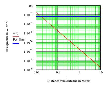
From the graph, it can be observed that the distance at which the RF exposure would exceed the limit would be approx. 2cm. The far field distance for a small antenna is given by any distance greater than  $\kappa/2\Pi$ ; this equates to a minimum distance of 5.3cm, therefore this calculation is not valid and so the minimum distance must be 5.3cm for which the calculation will become valid.
