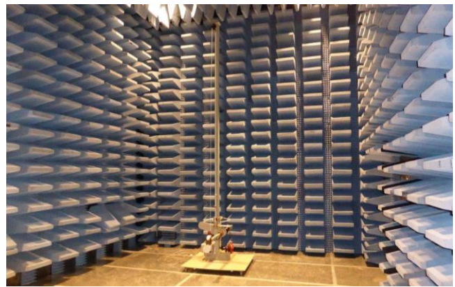
5 m Semi-Anechoic Chamber (SAC) in Everett, Washington
