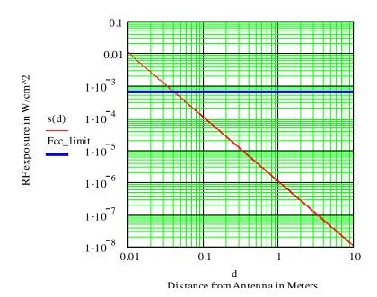
From the graph, it can be observed that the distance at which the RF exposure would exceed the limit would be approx. 4.2cm. The far field distance for a small antenna is given by any distance greater than  $\kappa/2\Pi$ ; this equates to a minimum distance of 5.3cm, therefore this calculation is not valid and so the minimum distance must be 5.3cm for which the calculation will become valid.
