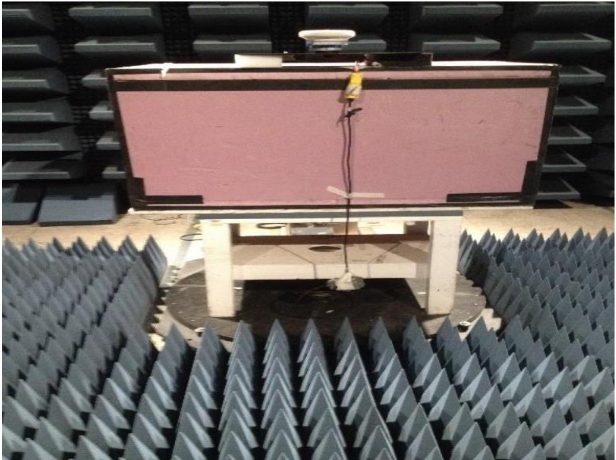
Emissions Test Setup – Unintentional Radiated Emissions 1000 - 10000 MHz (Close-Up view)
