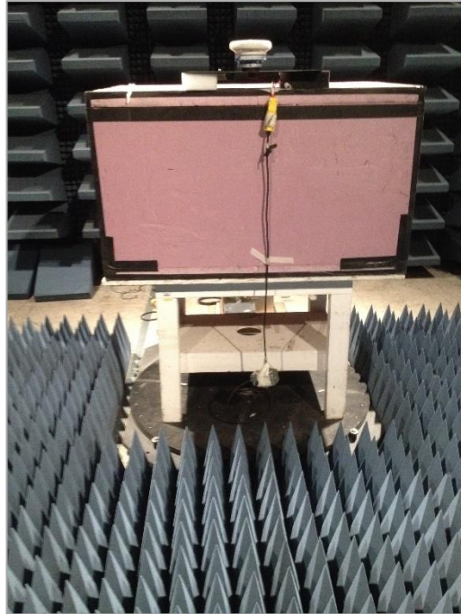
Figure 3: Radiated Emissions (close-up view) Test Setup
