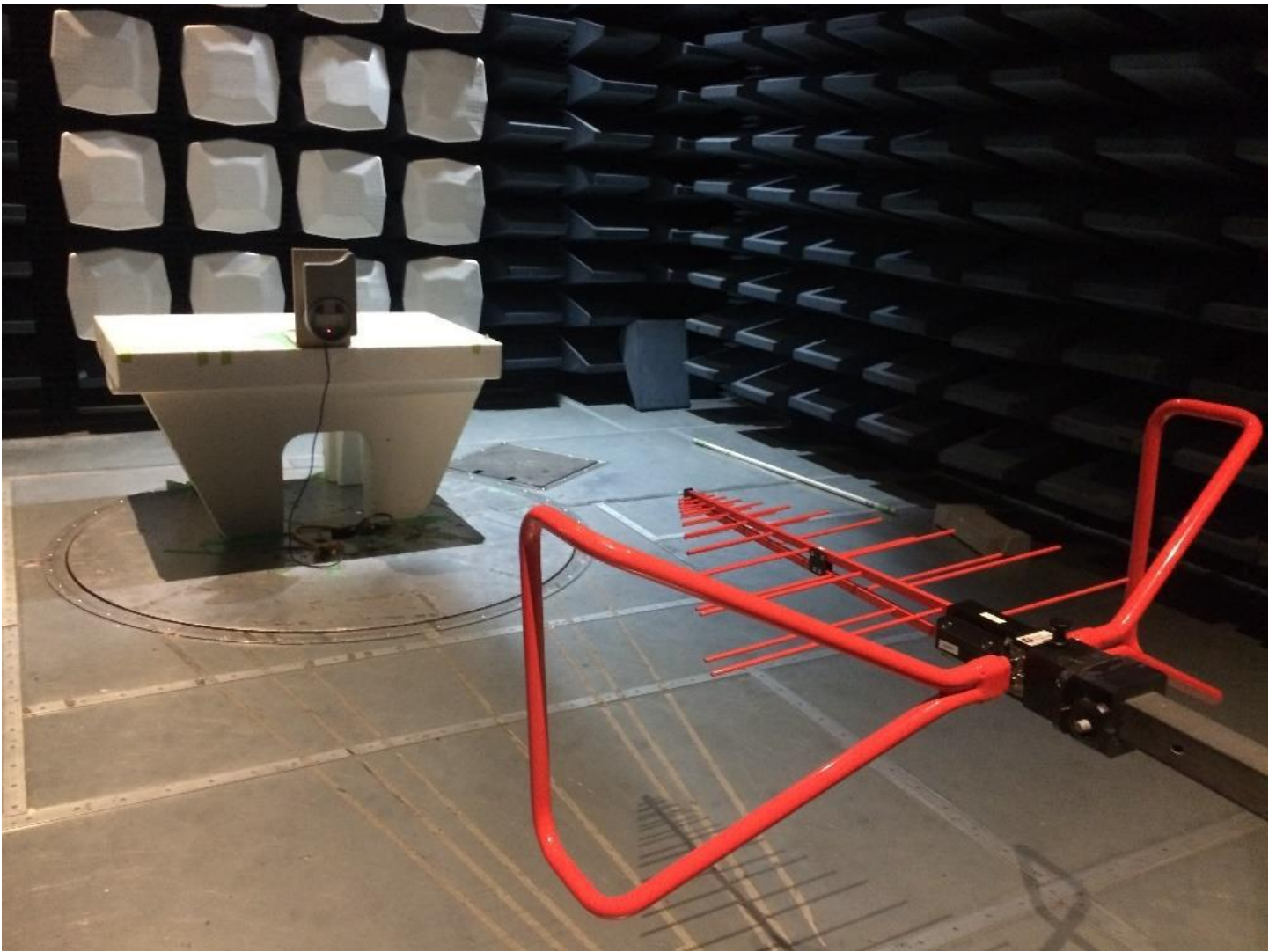
Emissions Test Setup – Unintentional Radiated Emissions 30 – 1000MHz
