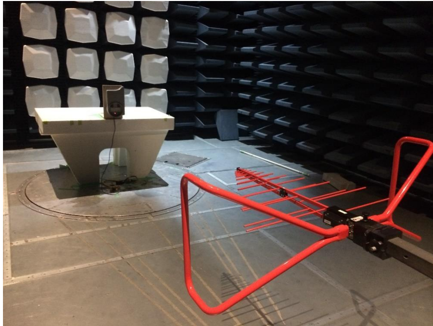
Figure 1: Radiated Emissions performed at the SAC Test
