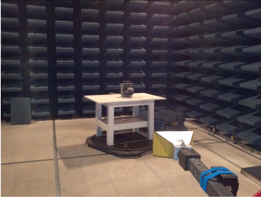
Emissions Test Setup – Intentional Radiated Emissions
