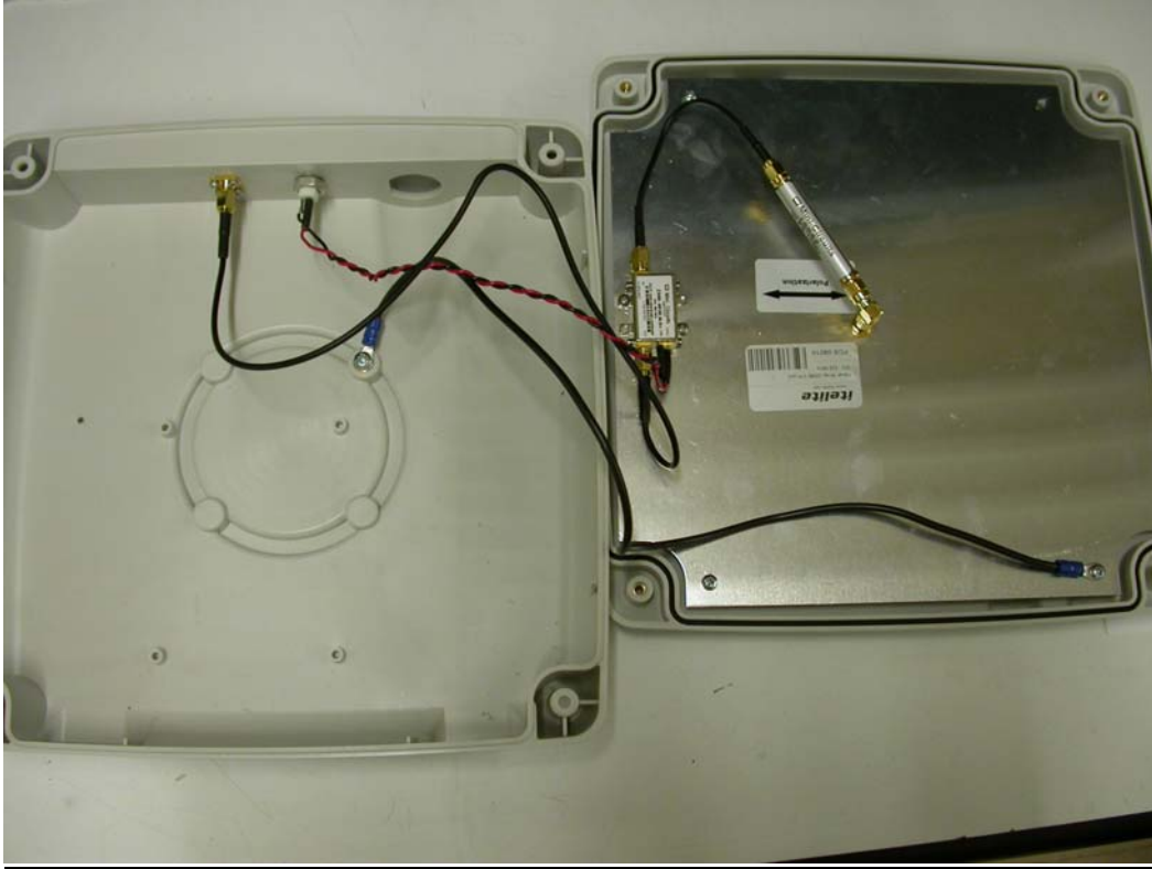
RX Antenna Internal View
