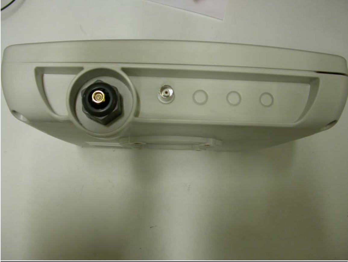
TX Antenna Connection View (Bottom)
