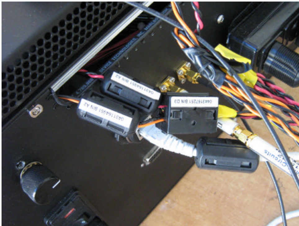
Figure 31 - Emissions Test Setup – Ferrites Added to Cabling
