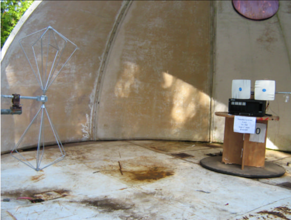
Figure 30 - Emissions Test Setup – Radiated Emissions
