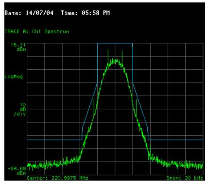
Measurement Results At The Lowest Channel 85% of primary supply voltage, 97 VAC
