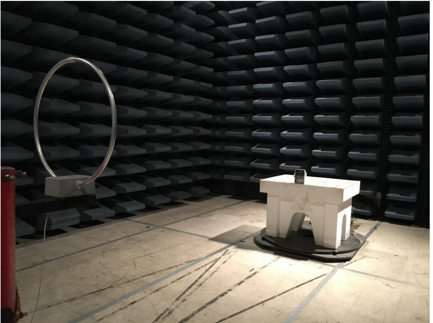
Emissions Test Setup – Unintentional Radiated Emissions below 30MHz
