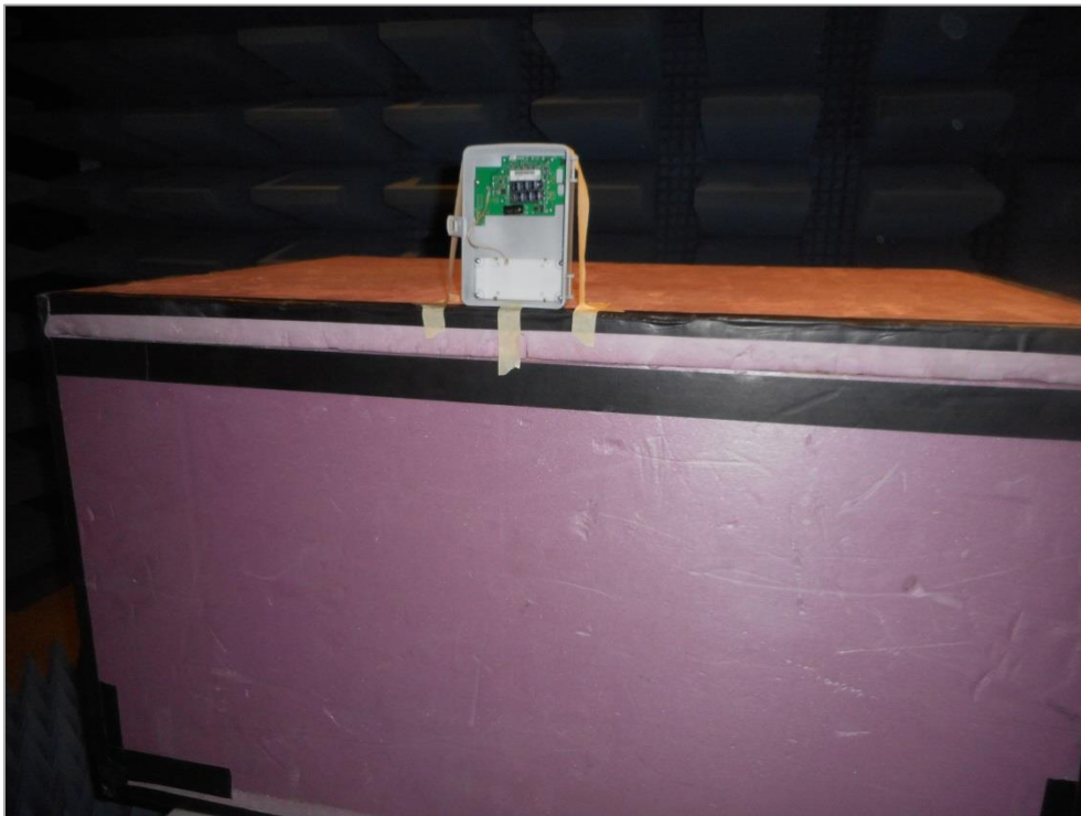
Figure 6: Radiated Emissions above 1 GHz performed at the SAC (close-up view) Test Setup
