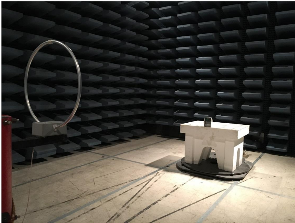
Figure 1: Radiated Emissions below 30 MHz performed at the SAC Test Setup
