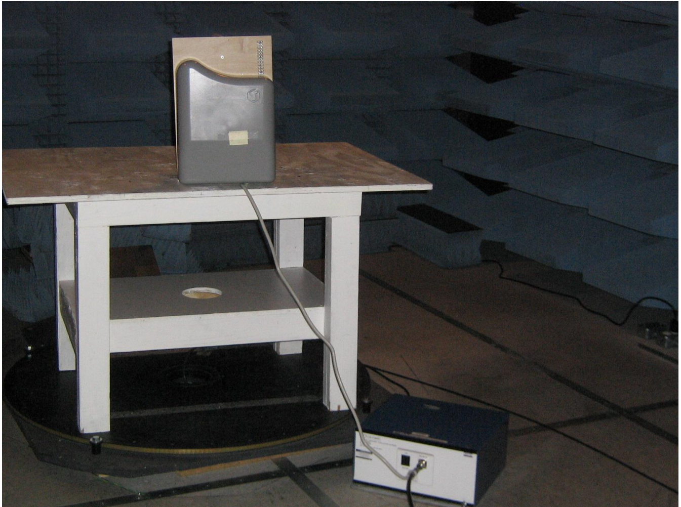
Figure 18: AC Conducted Test Setup
