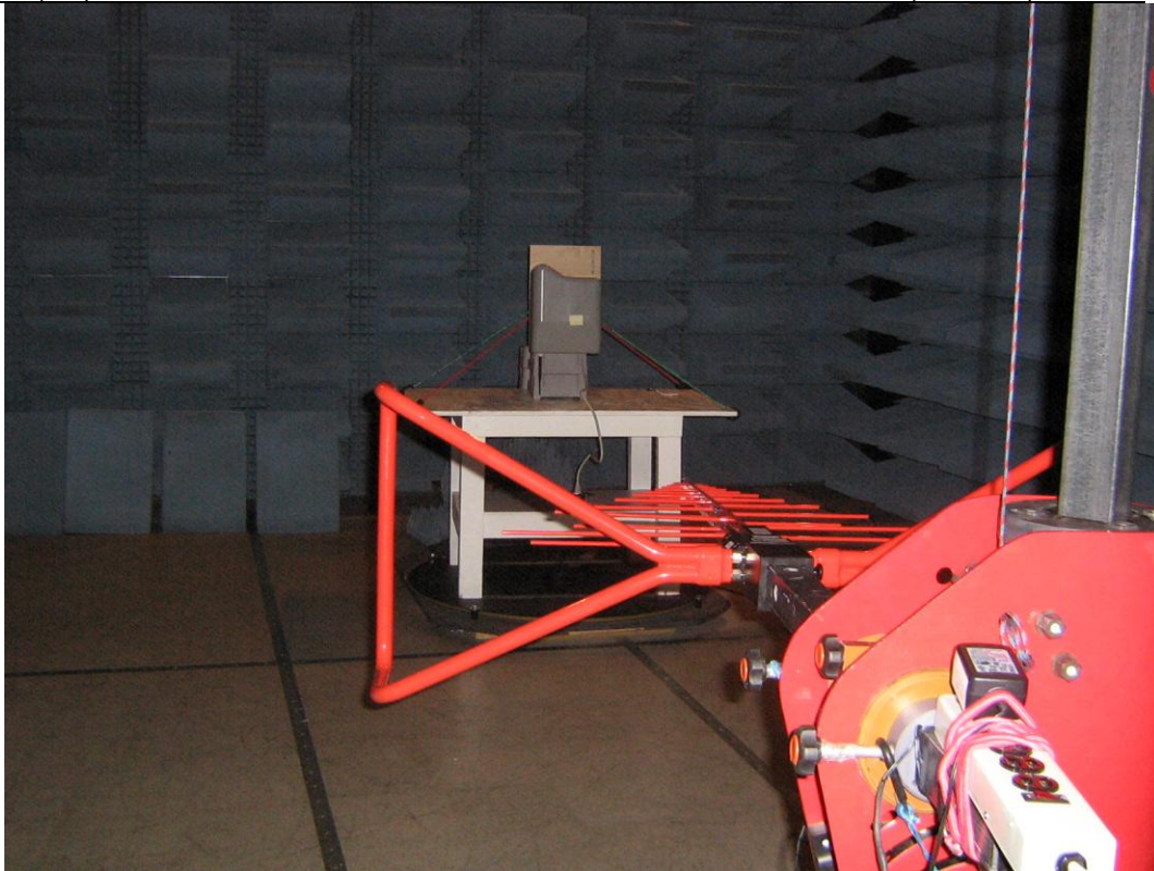
Intentional / Unintentional Radiated Emission 30 – 1000 MHz setup
