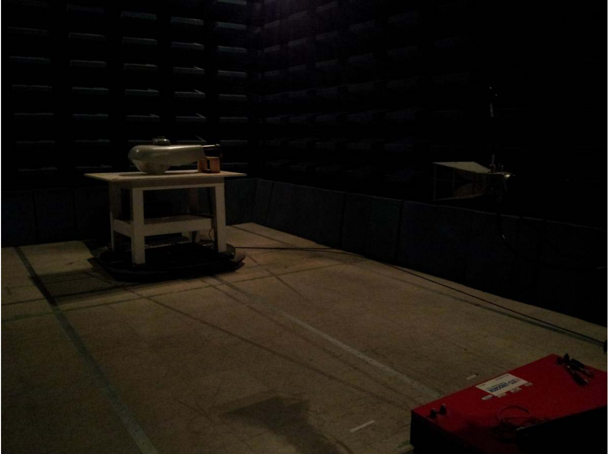
Emissions Test Setup – Intentional/Unintentional Radiated Emissions 1000 - 10000 MHz
