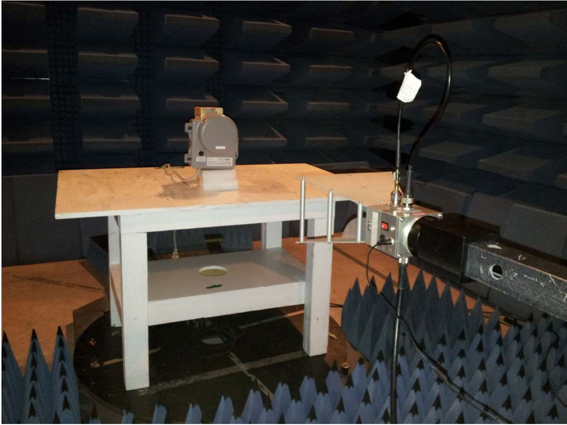
Emissions Test Setup – Intentional/Unintentional Radiated Emissions 1000 - 10000 MHz
