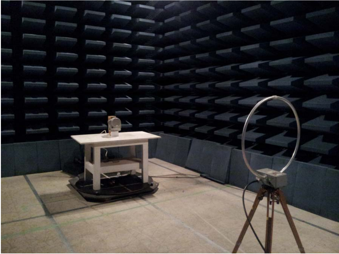
Emissions Test Setup – Intentional/Unintentional Radiated Emissions 0.009 – 30 MHz
