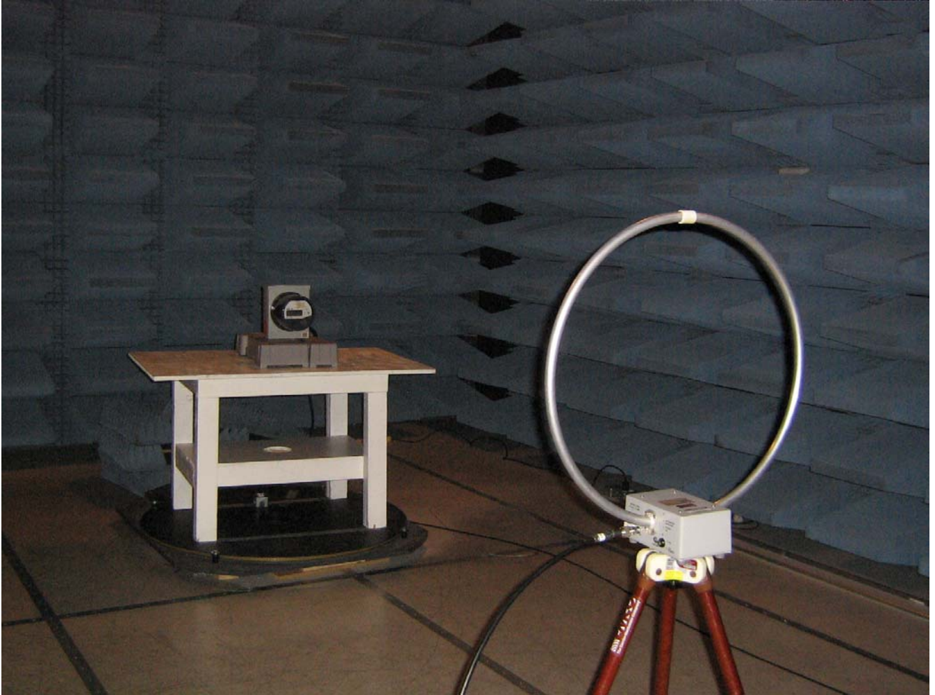
Emissions Test Setup – Intentional/Unintentional Radiated Emissions 0.009 – 30 MHz
